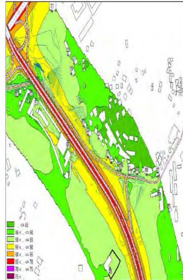
Figure 14 : Noise map calculated at 2m high – Situation 2021 with project, without noise barrier – Night period – West area
