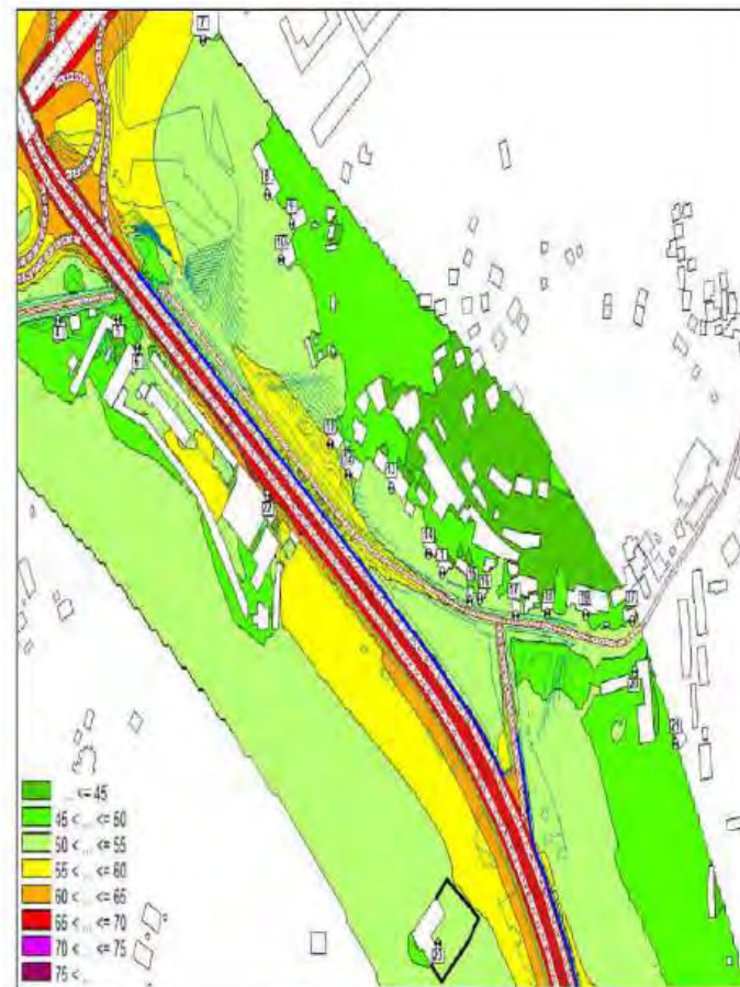
Figure 28 : Noise map calculated at 2m high - Situation 2030 with project, with noise barrier - Night period - West area
