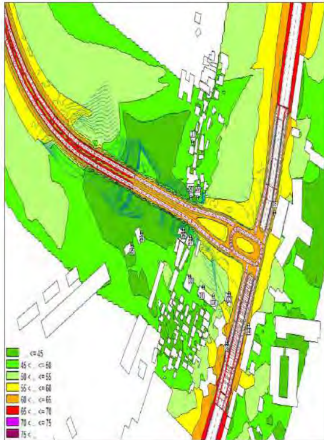
Figure 15 : Noise map calculated at 2m high – Situation 2021 with project, without noise barrier – Night period – East area
