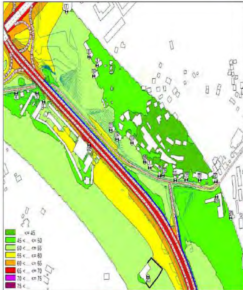
Figure 31 : Noise map calculated at 2m high - Situation 2080 with project, with noise barrier (v2) - Night period - West area
