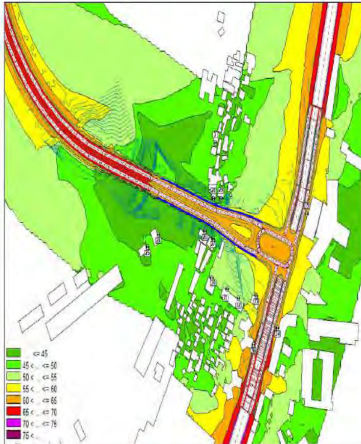
Figure 29 : Noise map calculated at 2m high – Situation 2030 with project, with noise barrier – Night period – East area
