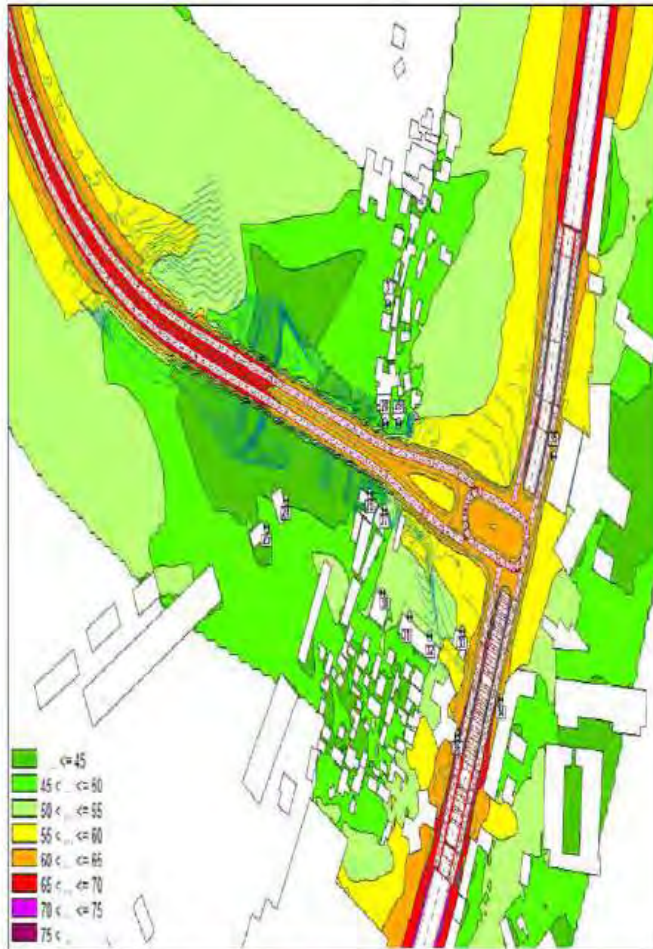
Figure 25 : Noise map calculated at 2m high - Situation 2030 with project, without noise barrier - Night period - East area
