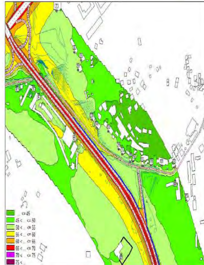
Figure 18 : Noise map calculated at 2m high – Situation 2021 with project, with noise barrier – Night period – West area
