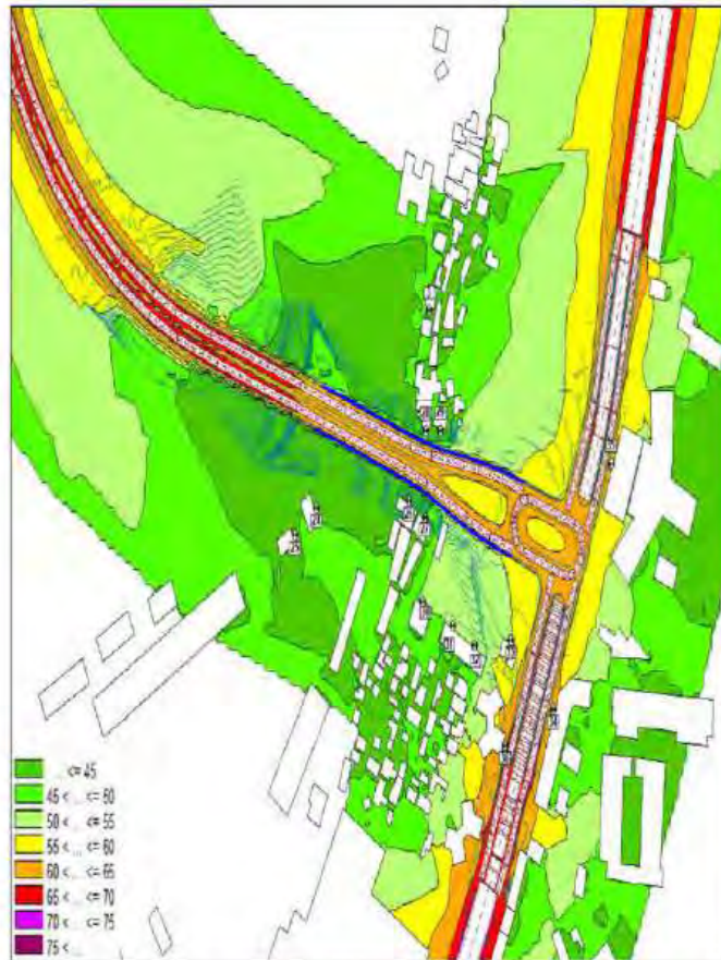
Figure 19 : Noise map calculated at 2m high - Situation 2021 with project, with noise barrier - Night period - East area
